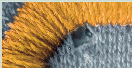
A needle point which is too sharp will create loop damage or needle cuts. A needle, which is too thick will push out the loop under tension and break it.
