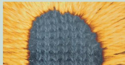
A DB x K5 size 65 with RG-point was used on this fine knitwear, the result is a nice embroidery design without any damage.
